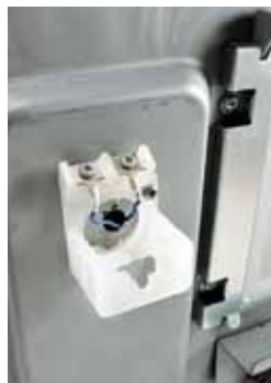
24VAC Terminal Block
